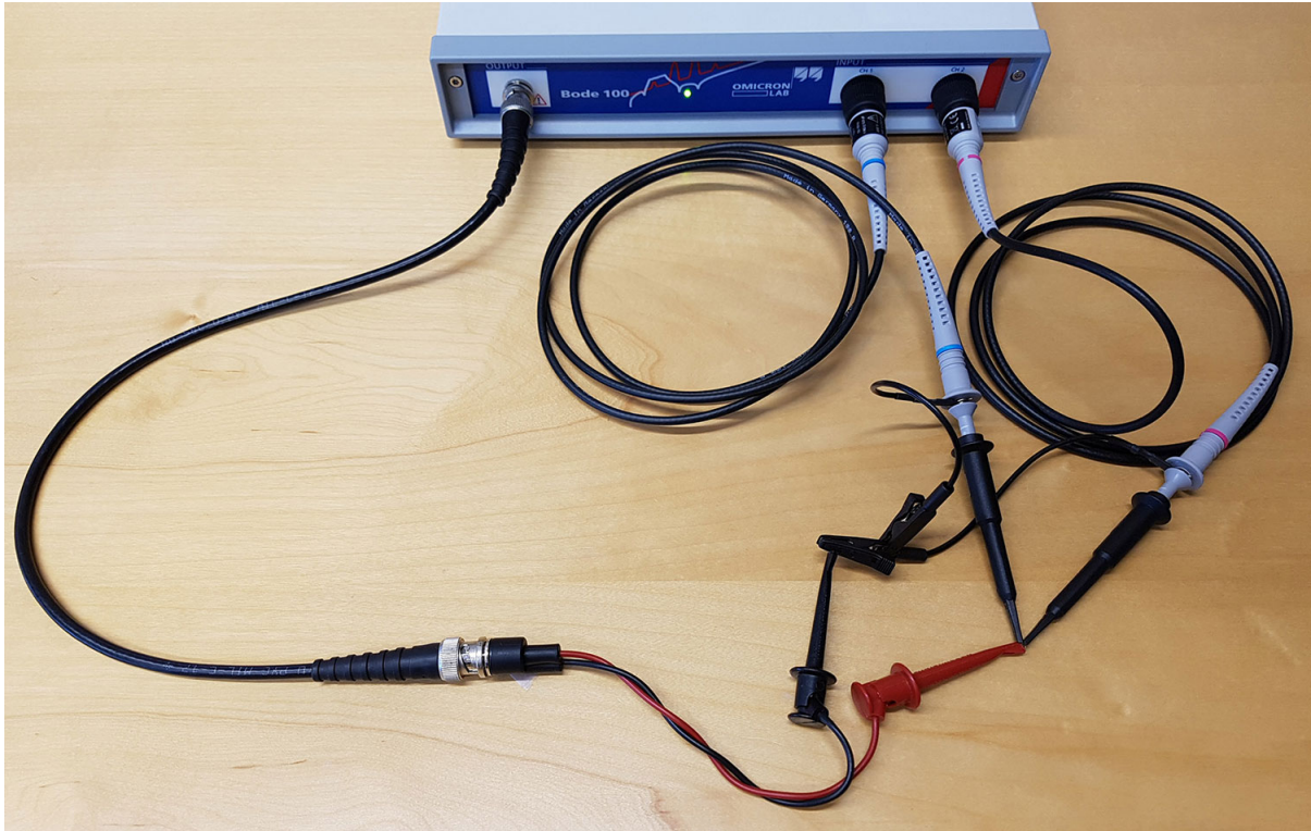
Figure 9-3: Typical Thru.calibration setup for gain/phase measurement using scope probes on Bode 100 .
